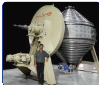
This Rota-Cone dryer from Paul O. Abbe is typical of vacuum drying equipment
