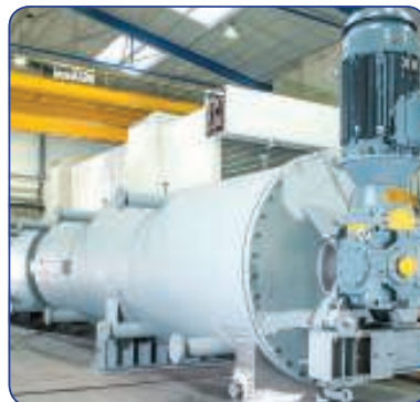
Indirect drying works well for many sludges and pasty materials
