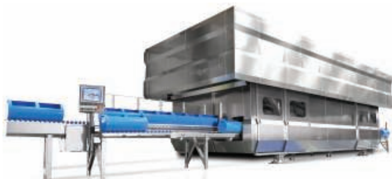
FIGURE 4. This high-pressure processor handles 3,000 kg/h
